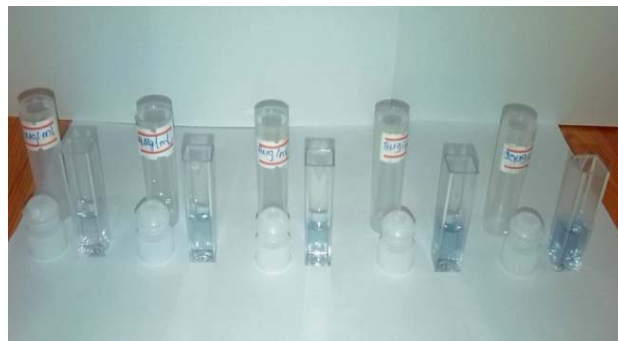
Figure 1: Prepared standard solutions of gallic acid with different concentration
