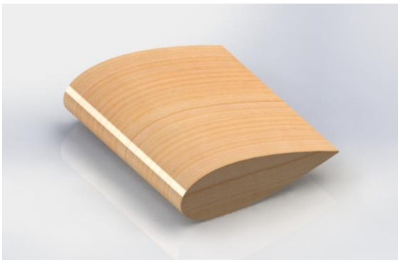
Fig. 1. 3D model of NACA 0012 profile
