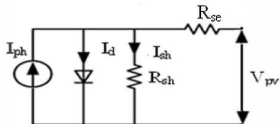
Fig 1. Equivalent Circuit for a Solar Cell
