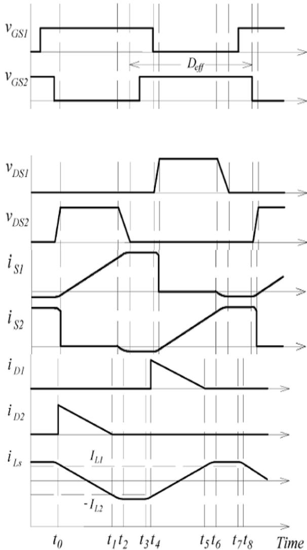
**Fig 3. Theoretical waveforms of Boost Converter**
