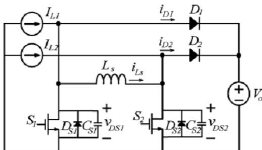
Fig 2. Proposed soft switching converter module
