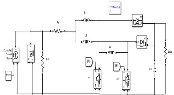
Fig 5. Simulink model of an Efficient Boost Converter
