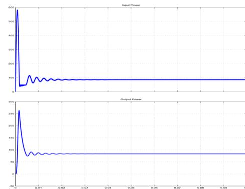
**Fig 10. Input Power 86W & Output Power 83.55W**
