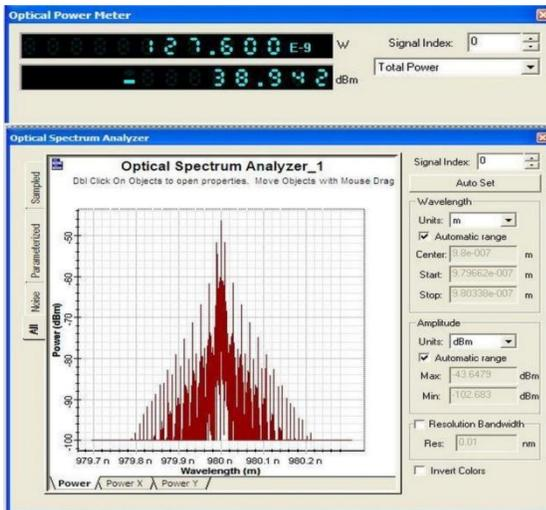
Fig. 7. Received optical power for link range 1700 km at wavelength 980 nm.
