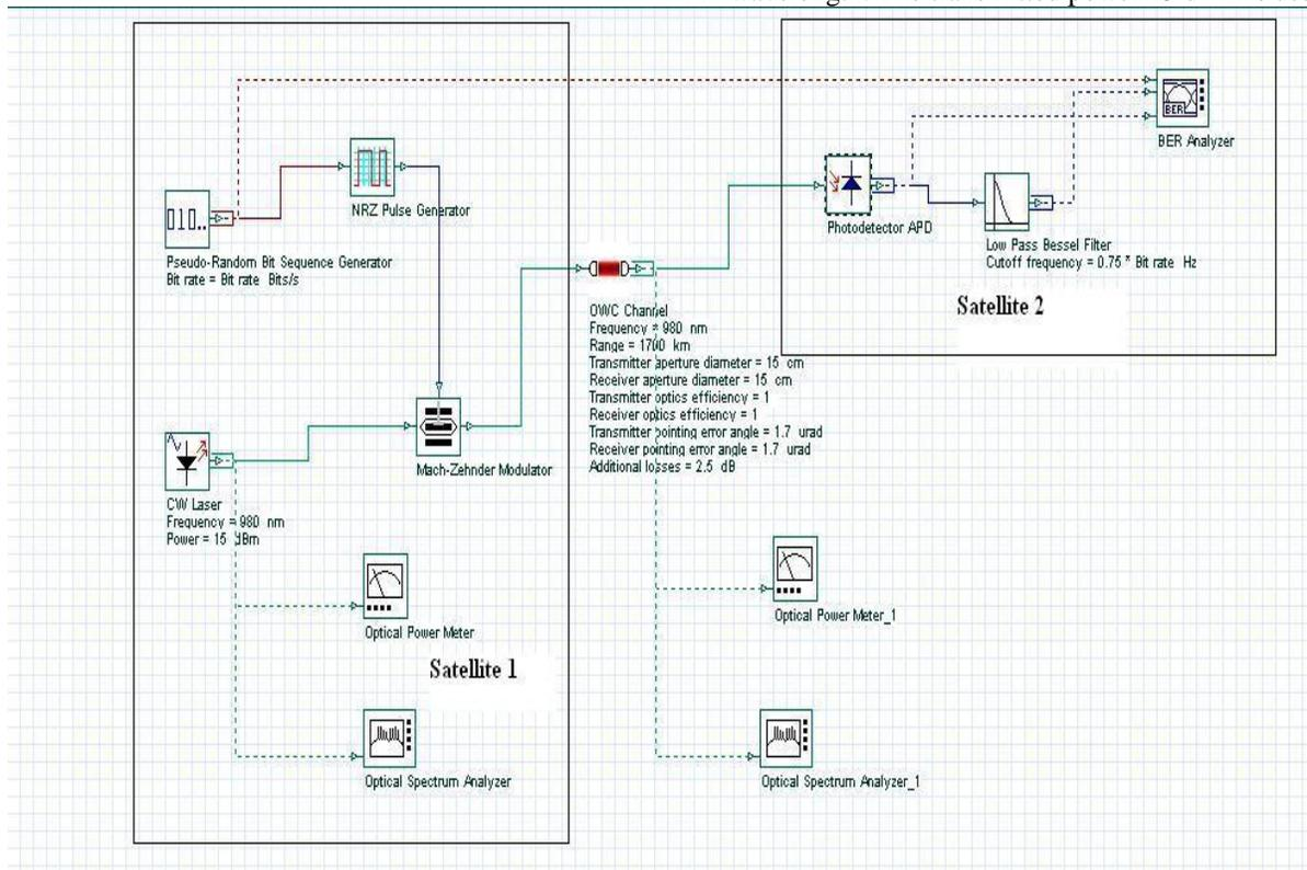
**Fig. 1 optimized IsOWC link using NRZ at wavelength 980 nm**
