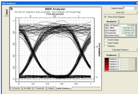
**Fig 3. Eye diagram of OWC inter-satellite system 1700 km apart with transmitting power of 15 dBm at operating wavelength of 980 nm by using NRZ.**
