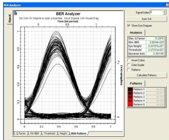
**Fig 6. Eye diagram of OWC inter-satellite system 1700 km apart with transmitting power of 15 dBm at operating wavelength of 980 nm by using RZ.**
