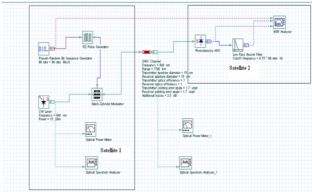
**Fig. 2. Optimized IsOWC link using RZ at wavelength 980 nm**
