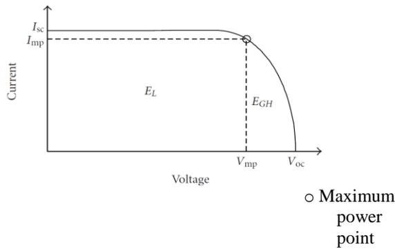
**Figure 2. Representation of a general I - V characteristic curve and its parameters.**
