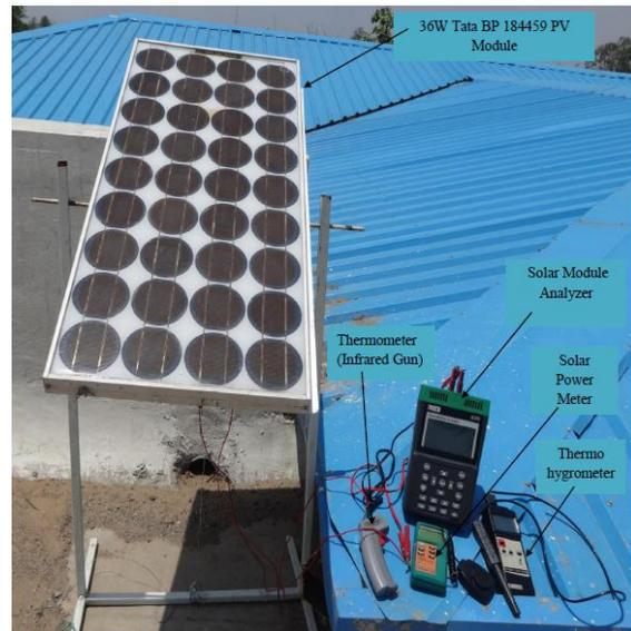
**Figure 3. Experimental set-up on the roof top at the energy center Maulana Azad National Institute of Technology Bhopal, India on 12 May 2014.**
