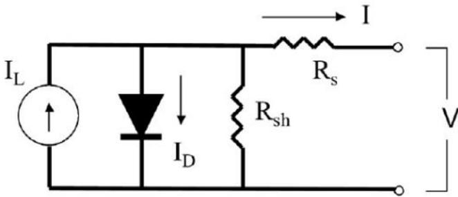
**Figure 1: Single diode model of a solar cell.**
