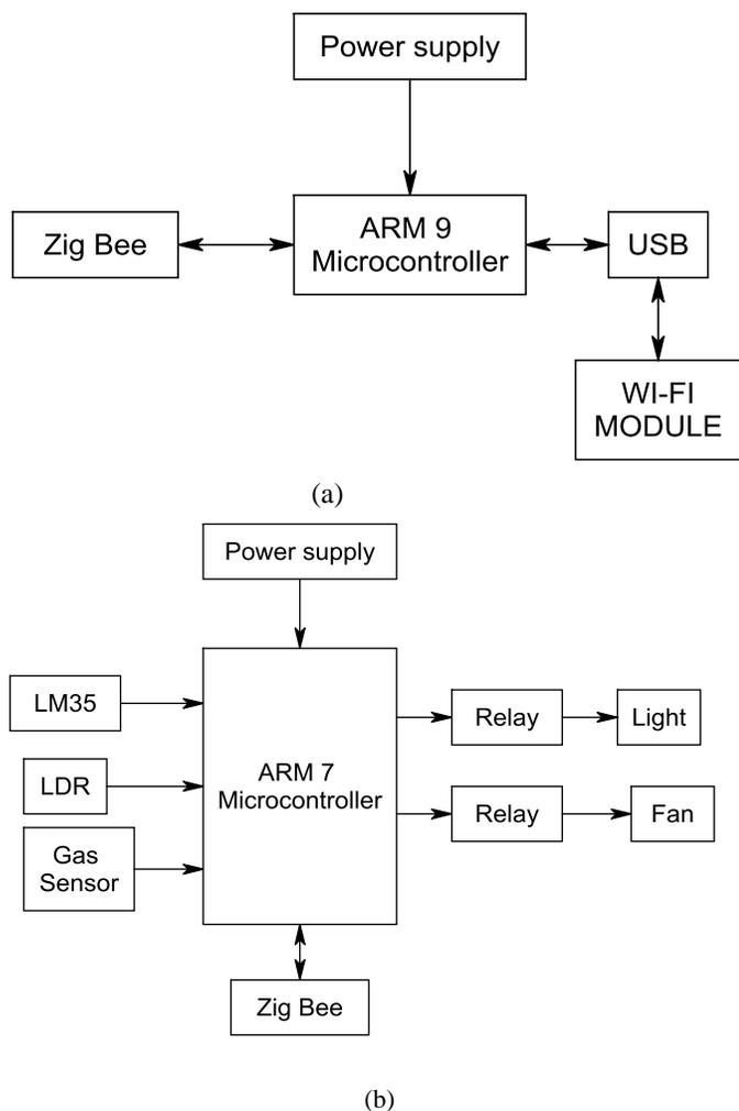
Figure 3: (a) Receiver Section (b) Transmitter Section
