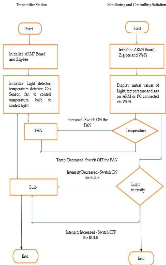
Figure 4: Flow chart for coal mine safety monitoring and control
