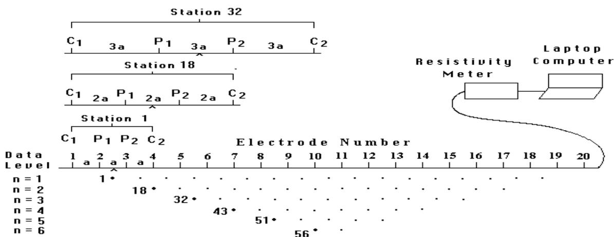
Fig. 3: Sketch of the electrodes for 2D geoelectrical resistivity survey and the sequence of measurement for building the pseudosection (Loke, 2011)
