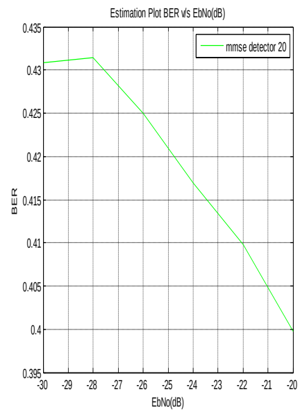
Bit Error Rate versus Average Signal to Noise Ratio For Linear CDMA MMSE Detector in Time Invariant Channel SIR = - 20dB
