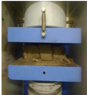
Figure 5.0: After Failure of Brick
