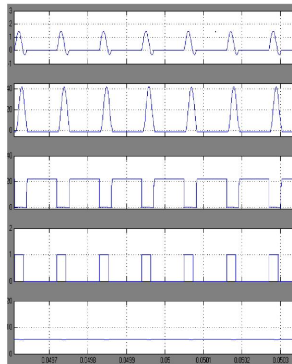
Fig 13: Simulation waveform (From top to bottom- resonant inductor current, resonant capacitor voltage, MOSFET voltage, Gate pulse, Output voltage)
