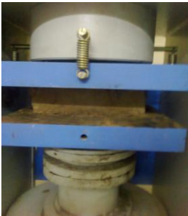
Figure 4.9: Before Failure of Brick
