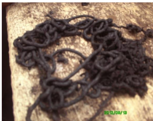
Figure: 6 Extruded bar before cutting to pellet size
