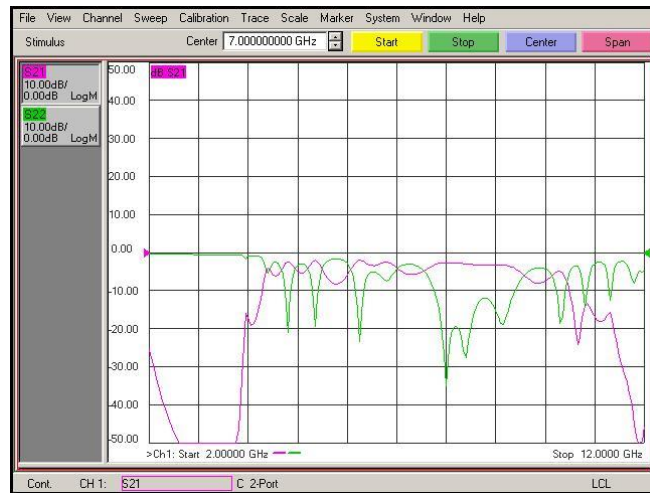
Figure 2. Measured results of reflectance and transmittance of a single ring microstrip filter
