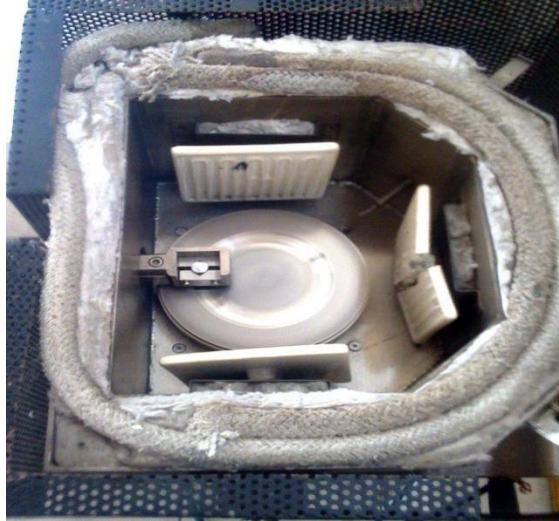
Fig.2 Pin on Disc wear testing machine TR20CH DUCOM
