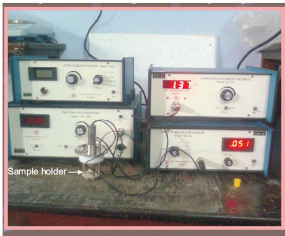
Fig 1 Four -probe set up.
