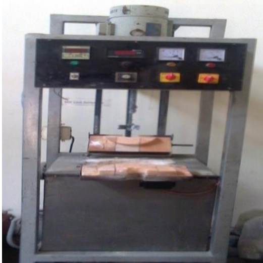
Fig.1 Stir Casting Setup
